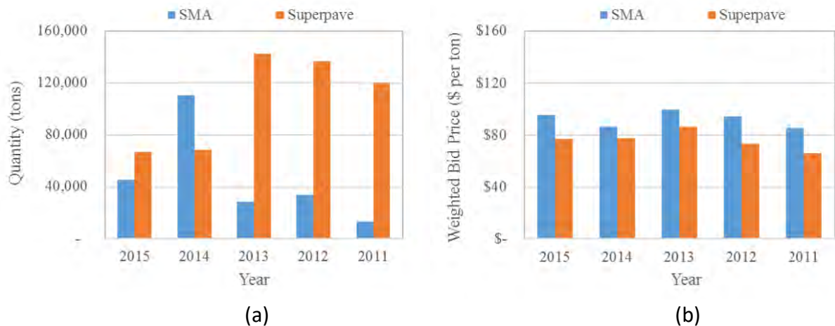
Figure A-9. Michigan DOT Information of SMA versus Polymer-Modified Superpave Dense-Graded Mixture; (a) Quantity, (b) Weighted Bid Price
