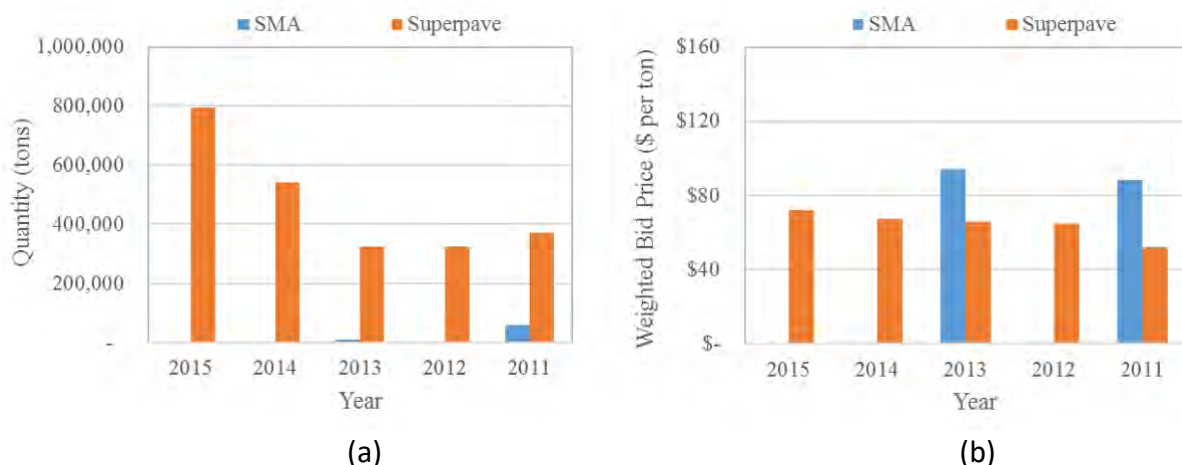
Figure A-7. Kansas DOT Information of SMA versus Polymer-Modified Superpave Dense-Graded Mixture; (a) Quantity, (b) Weighted Bid Price
