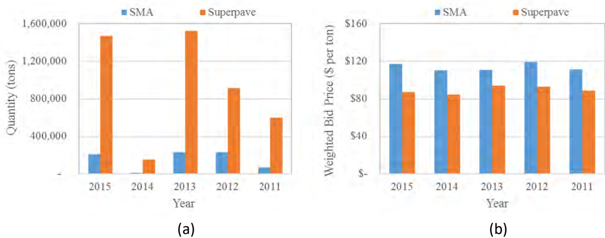
Figure A-12. Virginia DOT Information of SMA versus Polymer-Modified Superpave Dense-Graded Mixture; (a) Quantity, (b) Weighted Bid Price
