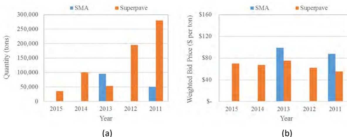
Figure A-10. Minnesota DOT Information of SMA versus Polymer-Modified Superpave Dense-Graded Mixture; (a) Quantity, (b) Weighted Bid Price
