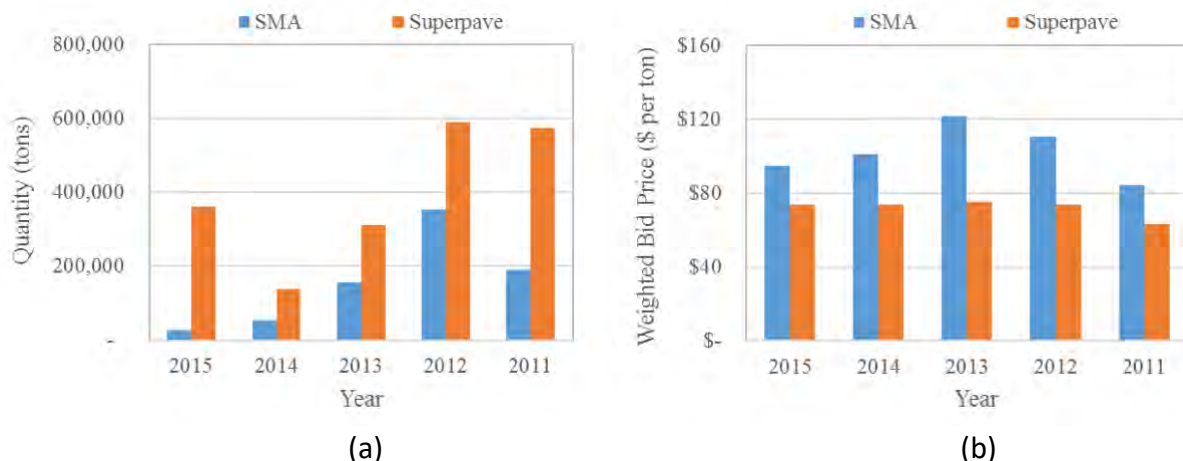
Figure A-3. Georgia DOT Information of SMA versus Polymer-Modified Superpave Dense-Graded Mixture; (a) Quantity, (b) Weighted Bid Price
