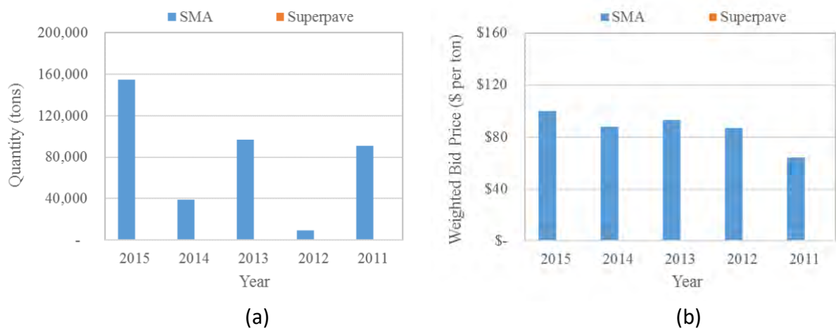
Figure A-13. Wisconsin DOT Information of SMA; (a) Quantity, (b) Weighted Bid Price
